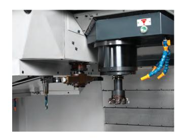
An integral ATC shutter separates the machine cutting zone from the tool magazine, assuring that chips and coolant from the machining area do not migrate into the tool magazine
