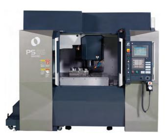
The chip and splashguard doors are strategically designed wider than the respective X – axis travel thereby insuring that full-size workpieces can be easily accommodated. In addition, the machine ceiling opens, together with the operator doors, to facilitate easy handling of large, heavy workpieces and fixtures that require an overhead crane.
