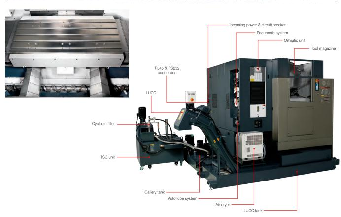
The chip and splashguard fully encloses the machining area to prevent flying chips and coolant from escaping outside the machine during manufacturing operations. The large, front operator windows provide outstanding visibility of the entire workzone.
